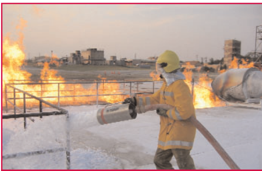
Medium expansion Tridol ATF foam controls LNG spill fire
